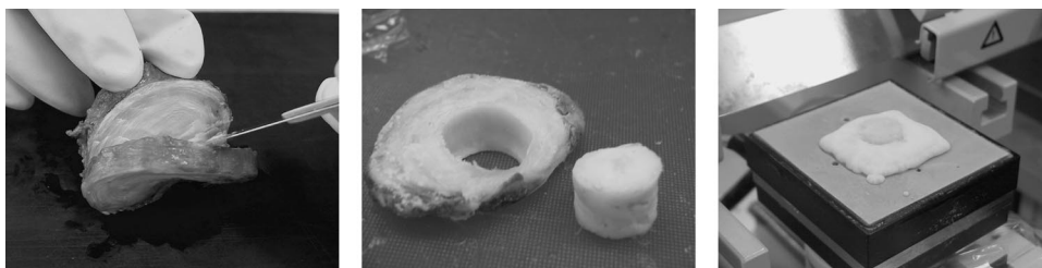
Figure 2. Preparation of human nucleus pulposus tissue for confined compression experiment. A cylindrical plug was removed from the center of the nucleus pulposus and microtomed to uniform thickness.
