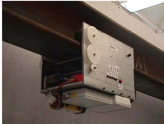
Figure 7 Beam Crawling Robot installed on laboratory I-Beam
